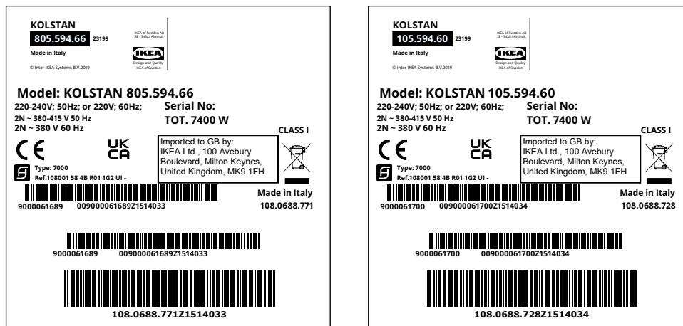
The graphic above represents the rating plate of the appliance. The serial number is specific to each product. Dear Customer, keep the additional rating plate attached to the cover of this booklet.
